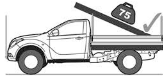
Reduce weight when inclined load. Recommended max overhang 10% of length.
