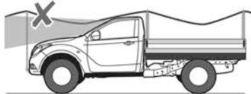
Driver's vision must not be obstructed. Flexible material may not be suitable on racks.
