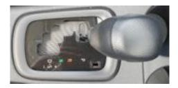
To change gears, simply hold the gear lever, push left and move down into the required gear and let go.
